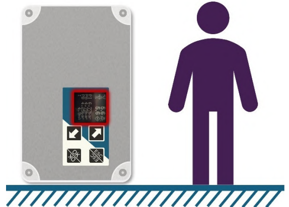
LUI WRONG ORIENTATION
