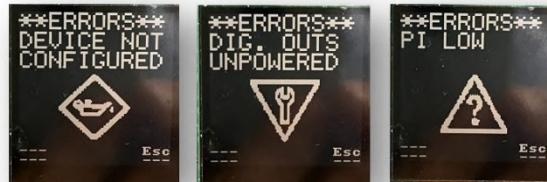
Figure 6 - Example of NE107 Active Alarms
