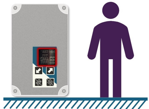
LUI WRONG ORIENTATION
