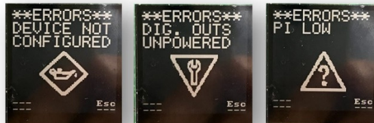
Figure 6 - Example of NE107 Active Alarms
