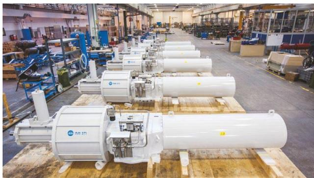
Quarter turn actuators for power & desalination project
