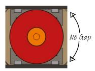
Our innovative Zero Backlash mechanism improves performance and solves the wearing-related gap issues between the sliding block and the scotch yoke slot, maintaining friction at similar levels to even the most established technology. It is available on request, please contact us for more information.
